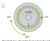
The Chafo has adjustable heat output. If a reduced heat is required, allow the Chafo to operate (in situ) at the MAX setting for approximately 30 minutes, then turn the Control Dial to any desired setting between MIN and MAX
