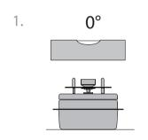
Put the Chafo on a level surface with the Burner Head uppermost
