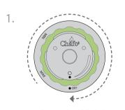
Rotate the Control Dial fully clockwise to turn off the Chafo
