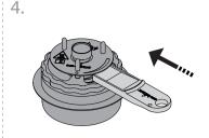
Reset the OTV device by carefully pushing the OTV Reset Tool between the Reflector Plate and Control Dial until it contacts the edge of the Reflector Plate
