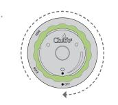
If the OSD has been activated, it must be reset before relighting. To reset, turn the Control Dial fully clockwise to the off position
