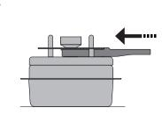
When cooled down reset the OTV with the OTV Reset Tool as described in Stage 1 before relighting
