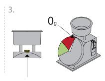
Zero the Scales by rotating the Zero Control Dial located below the Cradle. Find the OTV Reset Tool hanging at the side of Filling Station
