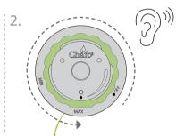
Turn Control Dial fully anti-clockwise. You will hear the fuel flow
