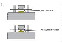
The OTV turns off the Chafo if the Vessel overheats. Always investigate and fix overheating problems before resetting and relighting
