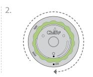
First reset the Chafo by turning the Control Dial fully Clockwise until it stops
